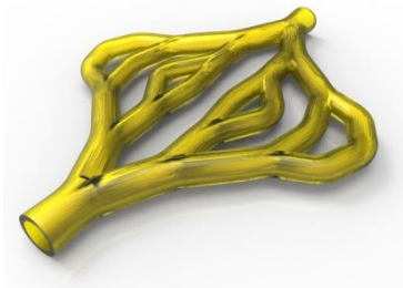
Figure 1: CAD solid model of optimized vascular system design.
