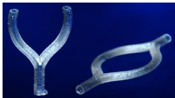
Figure 1: Tubes manufactured by stereolithography (Fraunhofer ILT)
